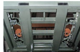
Bottom view of a big-bag filling station with vibrating system. The pneumatic cushioning allows dosing during vibrating. The weigher will not be affected by the vibrators. This system has a higher filling capacity compared to conventional vibrating units.
