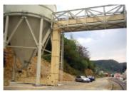
The continuous bucket conveyor is designed to transport bulk material from one or more infeed positions to a single high level discharge point. Continuous conveying without transfers can be achieved with horizontal, vertical or inclined configurations.
