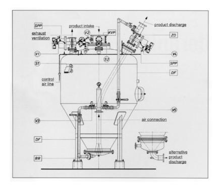
Pressure vessel DF: Pressure vessel for high pressure conveyance
