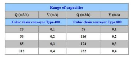
The conveying capacities are theoretical, calculated using a 100 % fill rate and 50 Hz.
