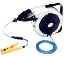
The **ground clamps** are designed for making and - in connection with **Terra-Control** ground system - for monitoring ground connections. The appliances are used in areas where potentially explosive materials and substances are loaded, discharged or refilled. Any developing static charges are safely and effectively eliminated and led to ground. This means that the risk of ignition caused by static discharges is eliminated at source.
