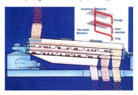
The model illustrated here is a typical two-surface machine, which separates material into three different grades. Other models have one to five screen surfaces, producing two to six separate grades.
