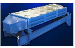
Screeners are self-contained production screening machines for separating dry materials according to particle size. Through their unique gyratory motion of the near-horizontal screen surface, combined with a positive screen mesh cleaning system, the screener provides unusually high efficiency and capacity - all the result of continuing development for hundreds of applications throughout scores of industries.
